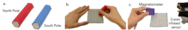
Figure 7: Imaging. (a) 3D printed magnetic pens. (b) Drawing a magnetic image onto a piece of magnetized fabric (c) Decoding the image by scanning a single magnetometer randomly around the image.
